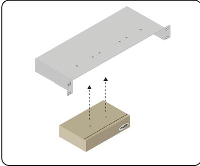
**Step 4** Install countersink screws.
