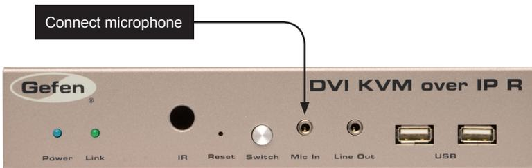
2. In order to get the audio from the microphone into the computer, connect a 3.5mm-to-3.5mm mini-stereo cable from the **Line Out** jack on the Sender unit to the **Line In** jack on the computer.
