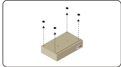
**Step 3** Line up holes on unit and rack tray.
