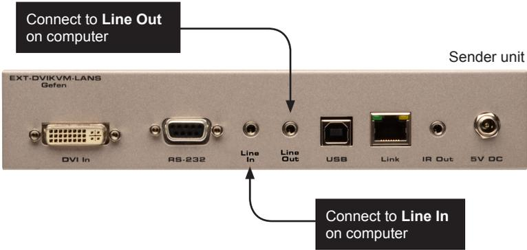
**NOTE:** When using HDMI sources with an HDMI-to-DVI adapter, the HDMI audio will be passed through to the DVI Out connector. However, if a 3.5mm-to-3.5mm mini-stereo cable is connected to the **Line In** jack on the Sender unit, the embedded HDMI audio is switched off. This allows the audio signal from the **Line In** jack (Sender unit) to be received on the **Line Out** jack (Receiver unit).
